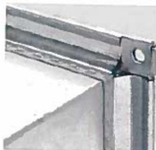
Cross flanges are obtained directly from the plate of the duct itself, avoiding the construction of the section frame to be fastened on duct. This technique represents an innovative goal in the cross joint system for rectangular section air duct: it allows a better airtightness, in compliance with the current provisions, and increases the mechanical resistance, which is fundamental during the installation and operation.
